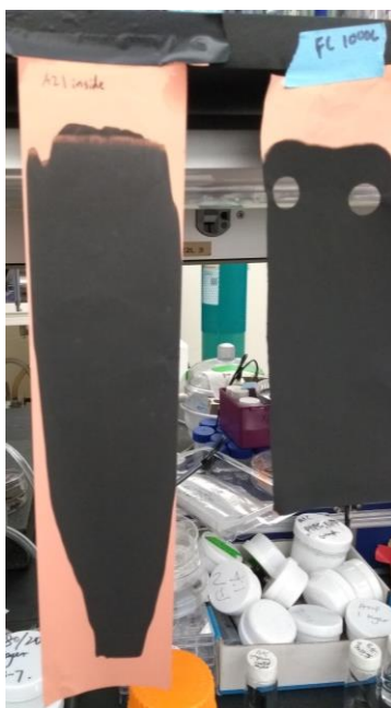
Figure 5. Copper foil piece coated with slurry made with carbon nanospheres, electrodes are cut out in circular shapes as can be seen in the right side piece
